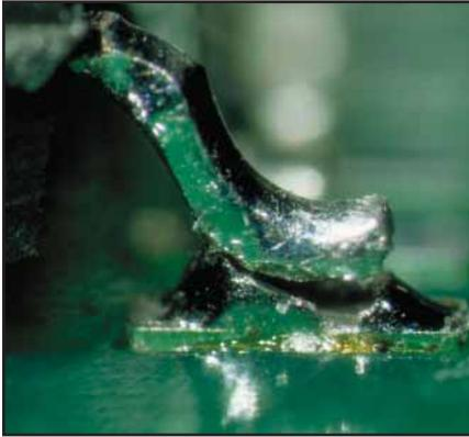
Fractured or cracked solder joint.
