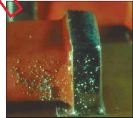
Typically small balls of the original solder paste that have splattered around the connection during reflow. If violating minimum electrical clearance, or not encapsulated, nor attached to a metal surface, then:
