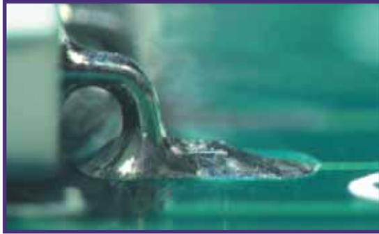
This photo represents an **ideal** surface mount solder joint for any class of Gull Wing component.
