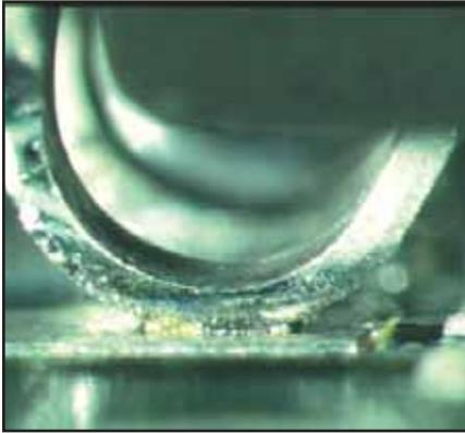
Solder fails to meet minimum fillet height. No evidence of properly wetted fillet.
