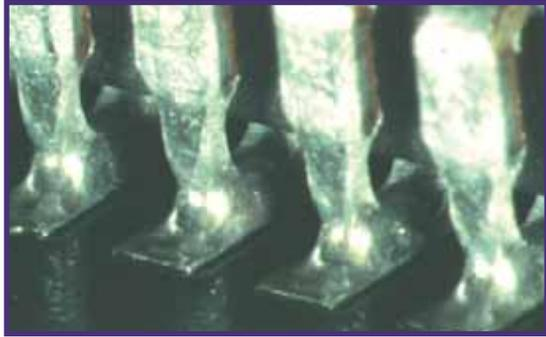
This photo represents an **ideal** surface mount solder joint for any class of J-lead component.
