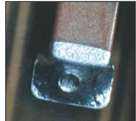
Larger holes (than pinholes) in the solder joint allowing voids, or trapped gases, to escape from the solder joint. Allowable condition as long as minimum soldering requirements have been met.
