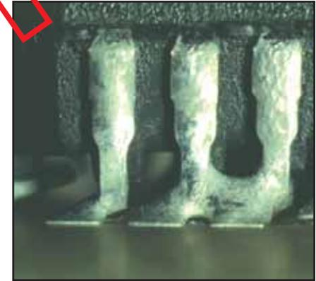
A connection of solder across conductors that should not be joined.
