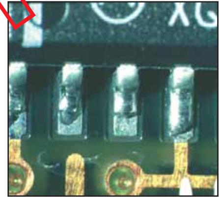
Molten solder coats surface then pulls back, leaving only a thin film of solder covering the land in some areas, and irregular mounds of solder in others.
