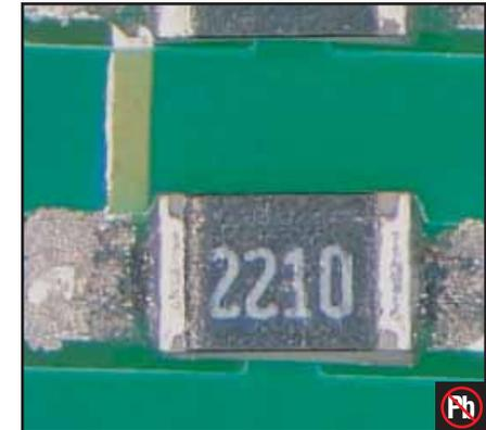
The solder paste had insufficient heat to reflow properly.
