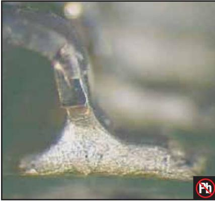
Lead free solder joints typically have a grainy or dull appearance.
