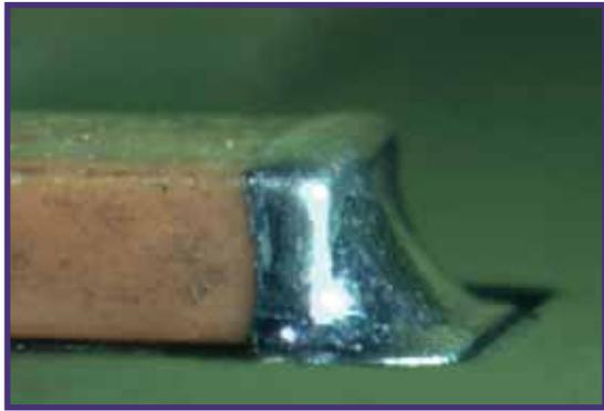
This photo represents an **ideal** surface mount solder joint for any class of rectangular chip component.
