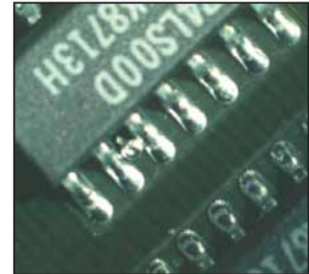
Any balls of solder that are not entrapped in a permanent coating, or attached to a metal contact, or violate minimum electrical clearance requirements.
