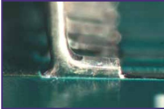
**Notes:** Solder joints are semi-transparent to show relationship between land and lead. Side Overhang, Dimension (A), must not violate minimum electrical clearance for assemblies with small (fine pitch) devices. Solder Thickness, or Dimension (G) is not specified for Class 3, only a properly wetted fillet must be evident. Please see Gull Wing, Class 1, for Dim. (G) picture. The references below are applicable to the dimensional criteria for Gull Wing components.
