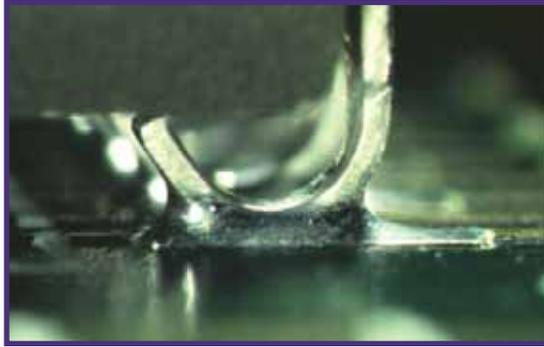
This photo represents an **ideal** surface mount solder joint for any class of J-lead component.
