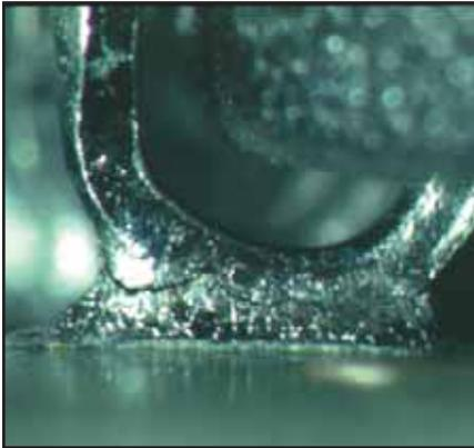
Fractured or cracked solder joint.
