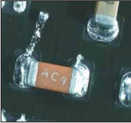
A film or splash of solder on any area that should be free from solder.
