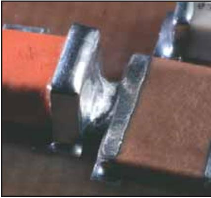
A connection of solder across conductors or lands that should not be joined.
