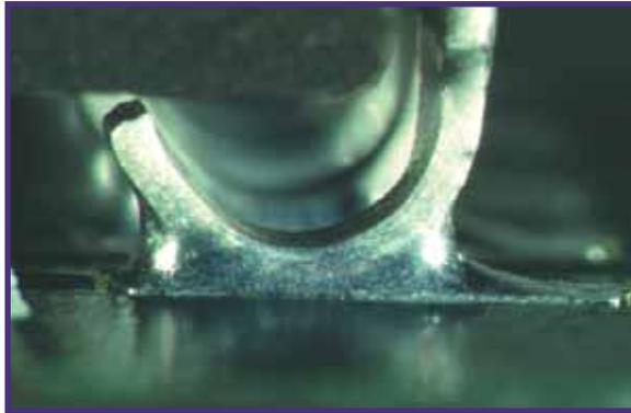
This photo represents an **ideal** surface mount solder joint for any class of J-lead component.
