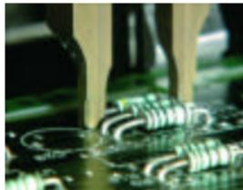
Axial inserter for through-hole components.
