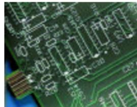
A printed circuit board with no components.
