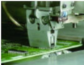
A DIP component insertion machine.
