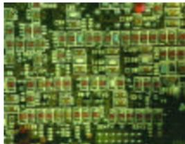
Chip components on the secondary side of the circuit board.
