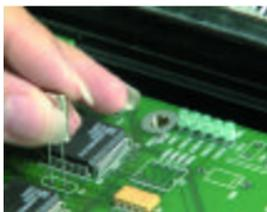
Manual insertion is used for some components.
