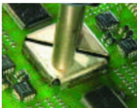
A rework hand tool removes the component.
