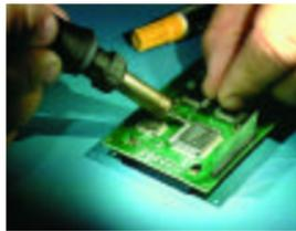
Reworking a bad solder joint.
