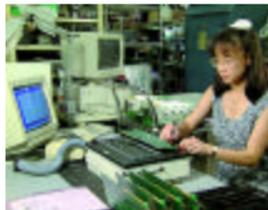
An assembly passes in-circuit test.
