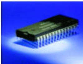
An IC in a Dual-In-Line Package.
